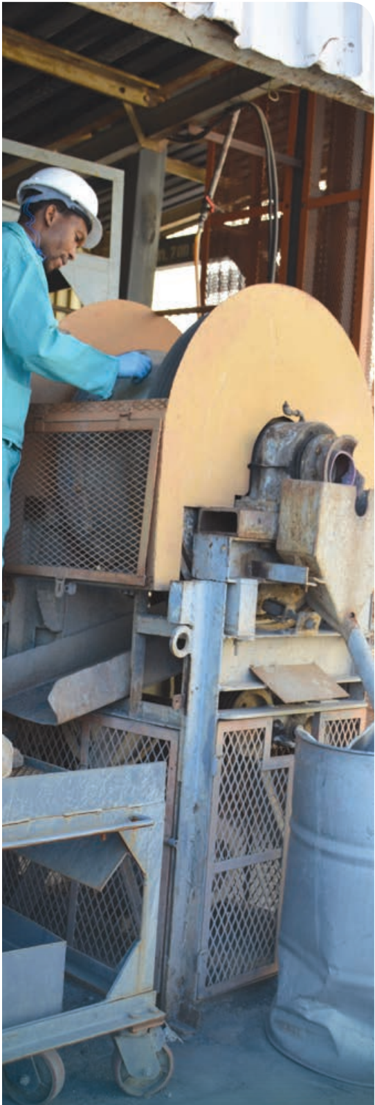
Experimental rubber lined ball mill (0.6m x 0.6m diameter) used to perform laboratory abrasive wear testing of different grinding media/balls from various suppliers, users (mines) and manufacturers.
