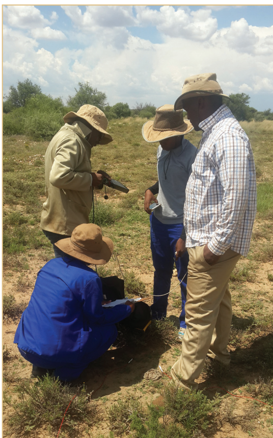
Setting up the hand-held acquisition computer for a time domain electromagnetic survey over a kimberlite target south of Reivilo, North West Province.
