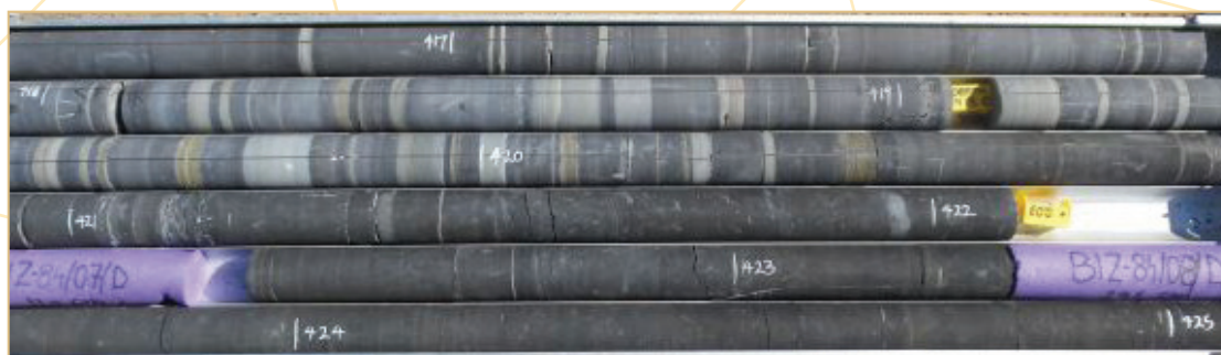
Dark-grey shale containing abundant lighter coloured tuff beds of the Collingham Formation overlying black carbonaceous shale of the Whitehill Formation at 420.46 m depth in the upper right of the core box. A sample of core has been removed for desorbed and residual gas analysis.
