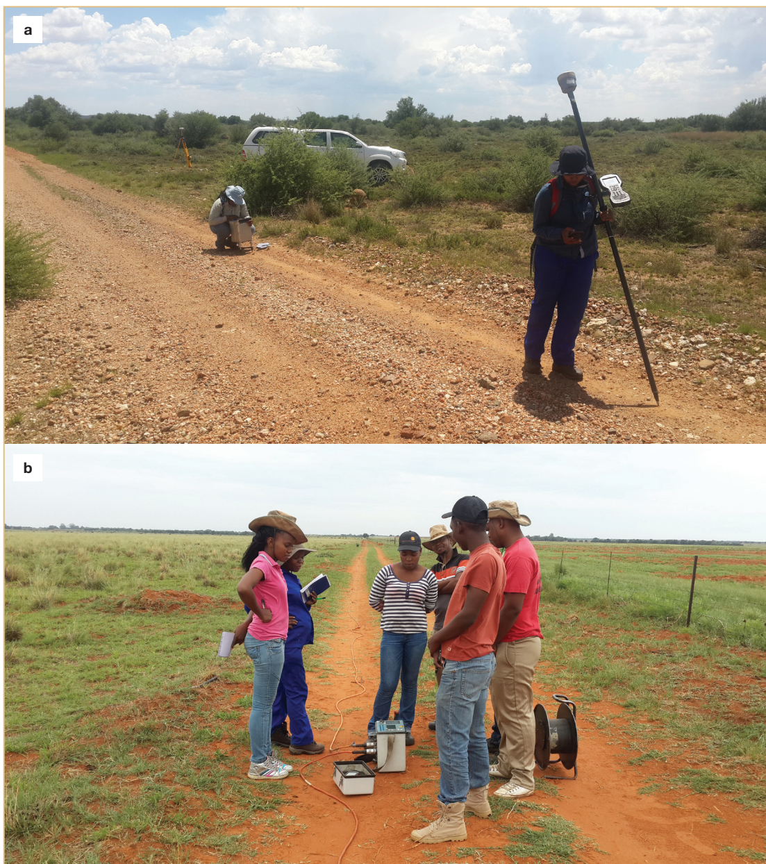
(a) Gravity survey across suspected Rietputs-type gravel channels near Windsorton, Northern Cape Province. (b) Electrical resistivity tomography survey for alluvial diamond exploration near Schweizer-Reneke, North West Province.
