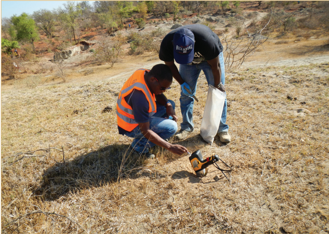
A handheld XRF spectrometer is used for in situ geochemical analyses.
