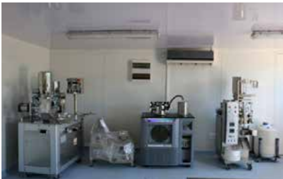
From left to right: Capsule-making machine, freeze-dryer, and teabag-making machine installed at the Agricultural Research Council's blueprint agro-processing facility for medicinal plants.
