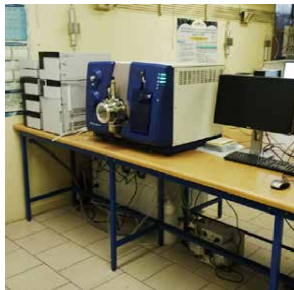
The newly purchased state of the art LC-MS/MS to be used to analyse synthetic steroids in serum and tissue
