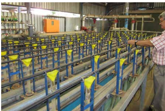
Inside the ARC irrigation laboratory – a researcher at the dripper test bench.
