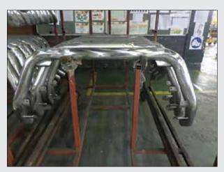
Figure 7: Part after 80% grinding
