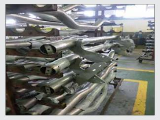
Figure 5: Before: Many parts get damaged after excessive grinding
