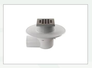
Seaqual F-Box WetFloor Drainage System is an integrated floor drainage system that consists of a number of components. These components comprise two sets. First set includes F-Boxes, waterproofing flange and round dust covers and the second set includes the M-sert, well, well cap, O-ring, grate and square protection cover.
