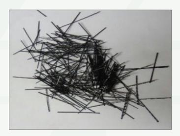
Geotex 500 and 600 series Macro-Synthetic Fibres are crimped, macro-synthetic fibers which are manufactured from a natural polypropylene homo polymer.
