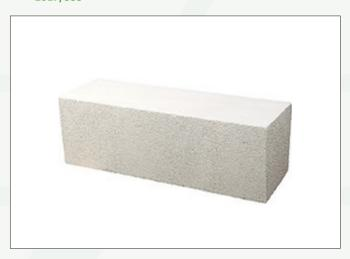
Everite Hebel Autoclaved Aerated Concrete (AAC) Block Building System is light-weight concrete masonry system. Blocks are factory produced from hydraulic binders (cement, lime & fly ash), fine sand, aluminium powder (expansion agent) and water.
